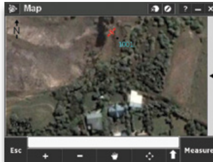
Above: A background image displays the location of the controller using the internal GPS and the point 1001 that you are navigating to.
