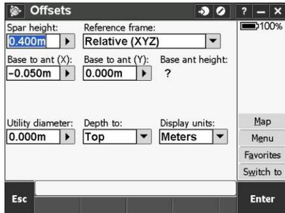
pole/tripod, then measure the distance from the mounting pole or tripod to the middle of the Spar’s handle. In the Spar’s coordinate system, forward means positive x, so the measurement you just made will be entered in “Base to antenna (X)” as a *negative* value (metric or US). Since the Spar is facing directly forward, the “Base to ant (Y)” value will be zero. Click “Enter.” (For more on offsets, see the Offsets video tutorial.)
